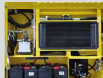
Heavy Duty Hydraulic Oil and Brake Cooling System
